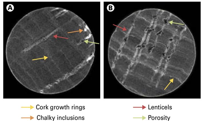
■ **Figure 3: Segmentation diagram of lenticels on 3D tomographic images based on segmented stoppers.**
